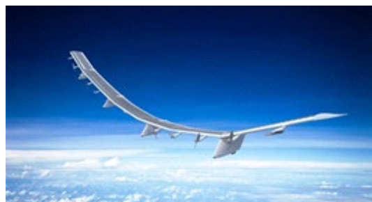
Figure 18: HapsMobile's Hawk30 High Altitude Pseudo Satellite
